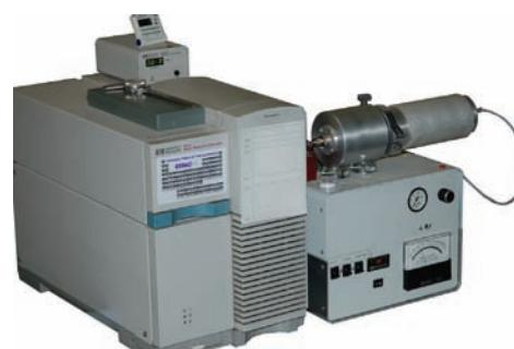
Figure 1 Genesis II particle beam interface.
